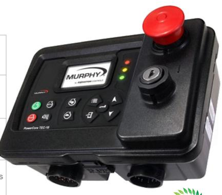
Murphy's PowerCore® TEC-10 panel provides full control of your engine including auto start/stop, auto throttling and display of engine parameters along with critical faults from the engine/application. The TEC-10 supports SAE J1939 CAN protocols for electronically governed engines as well as analog sensors on mechanical engines for fault and safety warnings/shutdowns.
